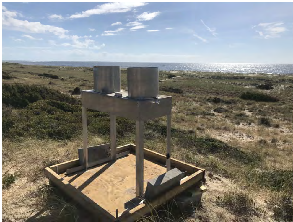
Fig. 3: Remote wet/dry deposition sampling station at Baldhead Island located on a 50 ft. dune ridge overlooking Cape Fear. This will allow collection of both wet and dry deposition samples representing a true marine air mass during certain wind directions.
